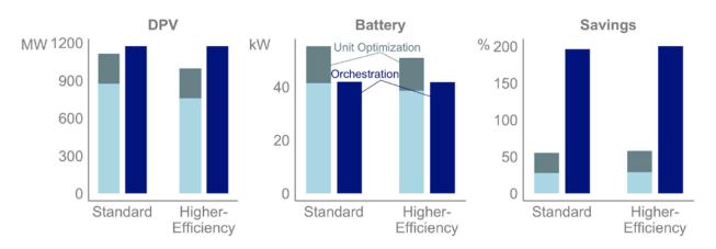
Figure 11. Modeled building energy system orchestration results for optimal DPV system size (left), battery size (center), and cost savings (right)
