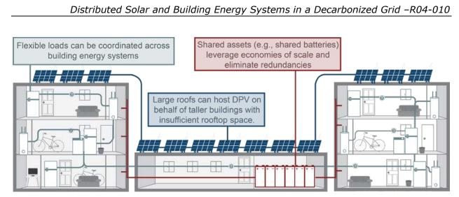
Figure 10. Schematic illustration of building energy system orchestration
