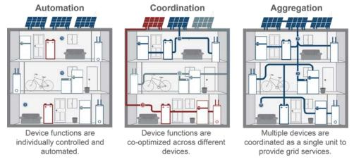
Figure 4. Building energy technology automation, coordination, and aggregation
